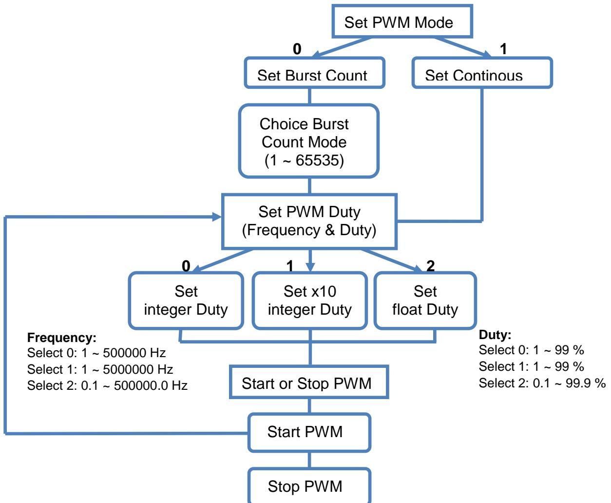
**Note:** Each time you change the settings of "PWM Duty", you have to re-send the "Start PWM" command to ensure the operation properly.
