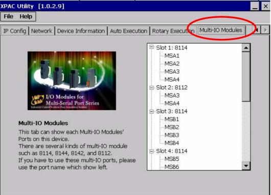
Step 2: The COM ports are grouped in the slot that the module plugged.
