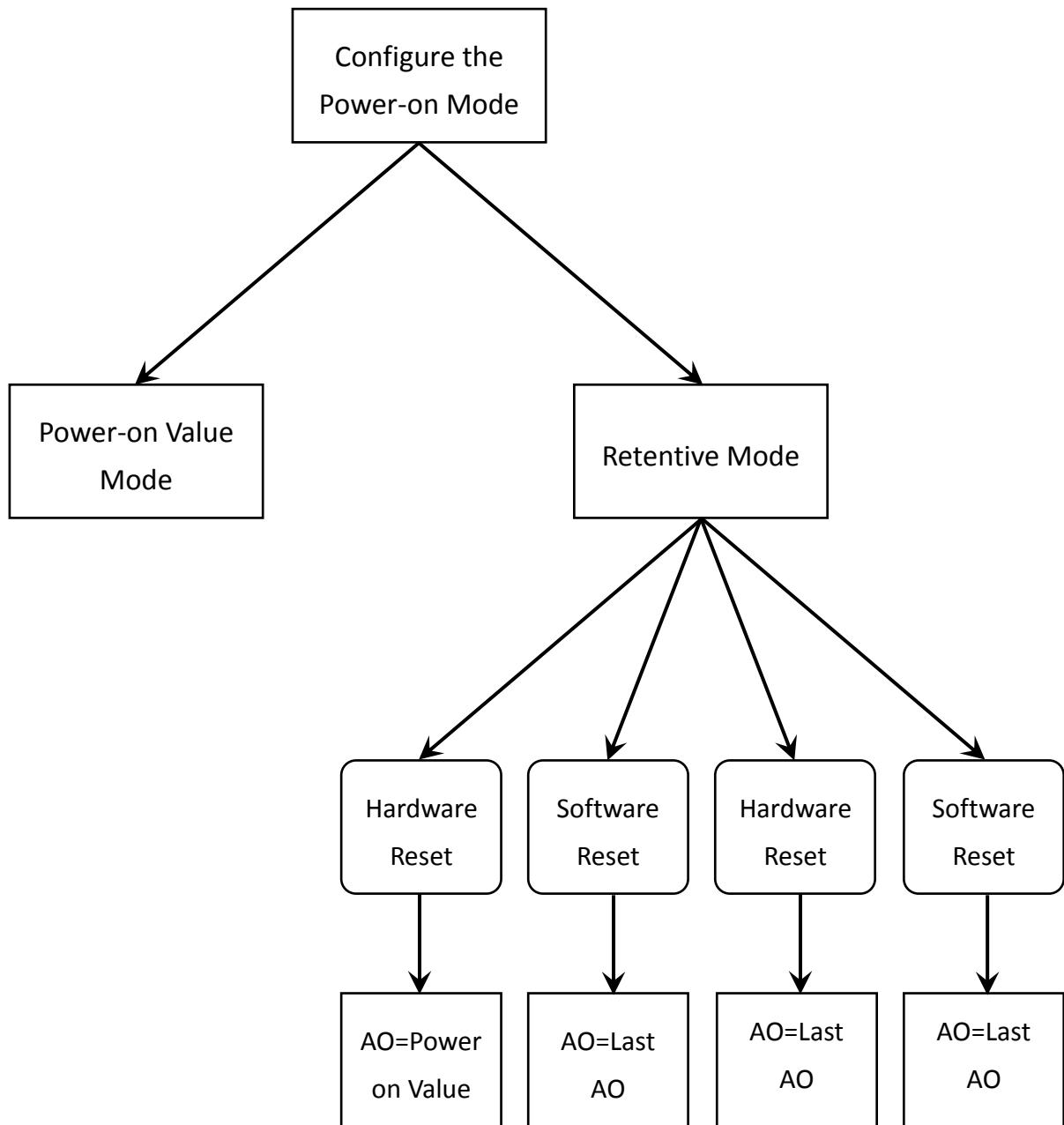
Note: the term Previous AO value means that the AO value that was active prior to the reset will be retained. For example, if the Power-on Mode is set as Retentive Mode and a hardware reset occurs, then the AO value will be the same as the value that existed prior to the hardware reset.
