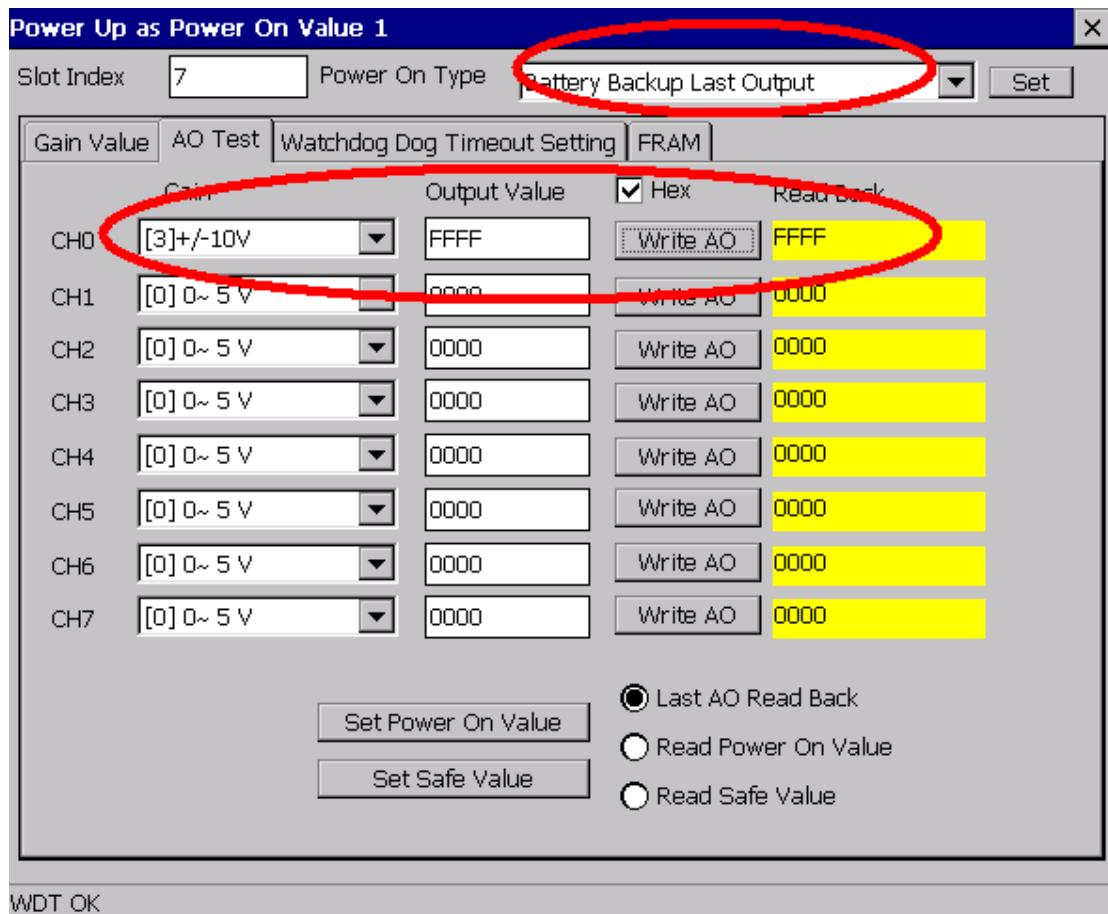
After the power to the 9000-series PAC is reset, the AO value for channel 0 will be Gain 3 (+/-10 V) and the Output value will be set to 0xFFFF, as Illustrated in the figure below.
