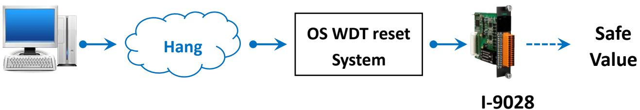
To set the WDT on the 9000-series PAC to enabled, use the `pac_EnableWatchDog(intwdt, DWORD value)` function and set the value attribute to 0.
