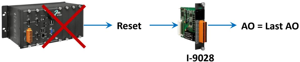
For example, set channel 0 on the I-9028U module to Gain 3 (+/-10 V) and the Output value to 0xFFFF in Retentive Mode.
