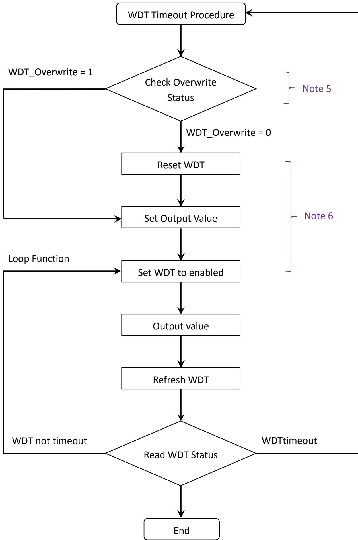
If a Watchdog timeout occurs and the WDT\_Overwrite parameter = 0, all the Analog Output values on the I-9028U will be switched to Safe Values, and any operations where an output value needs to be written will not be accepted until the Watchdog is reset. In contrast, if a timeout occurs and the WDT\_Overwrite parameter = 1, any output value that is written will be accepted and will reset the Watchdog.
