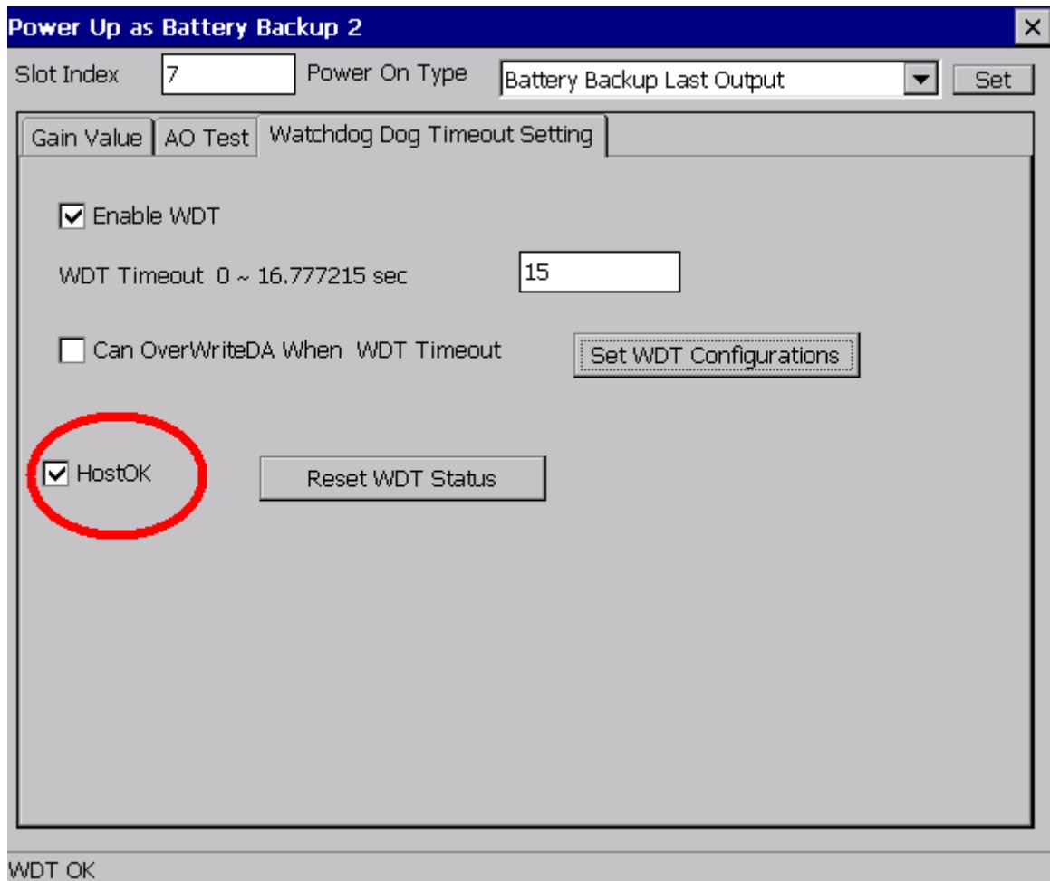
If the HostOK checkbox is checked, the status of the module will be regularly polled to and the pac\_i8028U\_RefreshModuleWDT function will be executed to refresh the WDT, ensuring that a WDT timeout will not occur.
