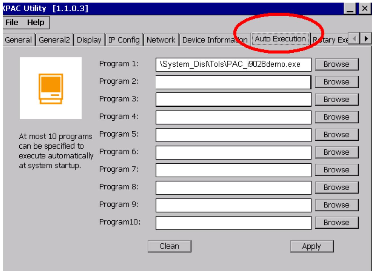
By using a combination of the Auto execution function in the XPAC Utility and the Power-on Mode function on the I-9028U module, the stability of an application's performance can be improved.
