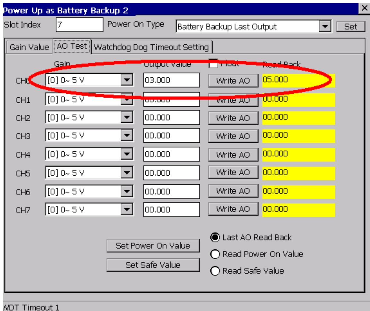
The WDT timeout and the AO switch to the Safe Value of 5 V.
