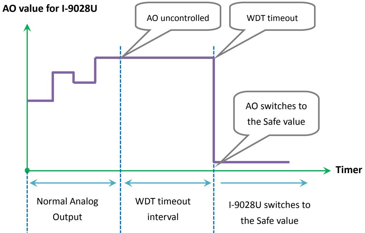
Watchdog operations include basic management operations, such as turning on and refreshing the module. The following sections provide a description of how to programmatically operate the watchdog using the watchdog functions.
