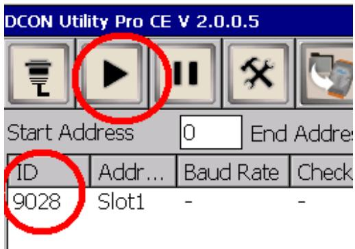
4. Use the DCON Utility Pro to configure the parameters for AO, Power-on Mode, WDT and others to quickly test all the I-9028U functions, as illustrated in the example below
