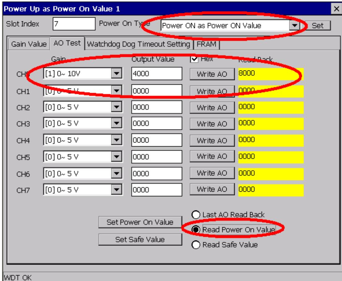
After the power to the 9000-series PAC is reset, the output value for channel 0 will be Gain 1 (0~10 V) and the output value will be set to 0x7FFF, as illustrated in the figure below.
