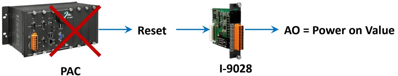
For example, set the Power-on Value for channel 0 on the I-9028U module to Gain 1 (0~10 V) and the Output value to 0x8000 in Power-on Value Mode, but the output value is 0x4000.
