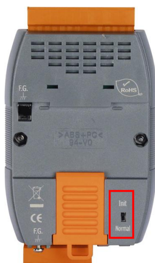
Figure 2-1 : The switch is located at the back of the controller
