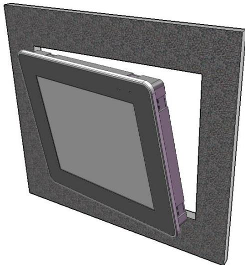
**Step 3: Insert the panel mounting clips into the upper and lower ventilation holes**
