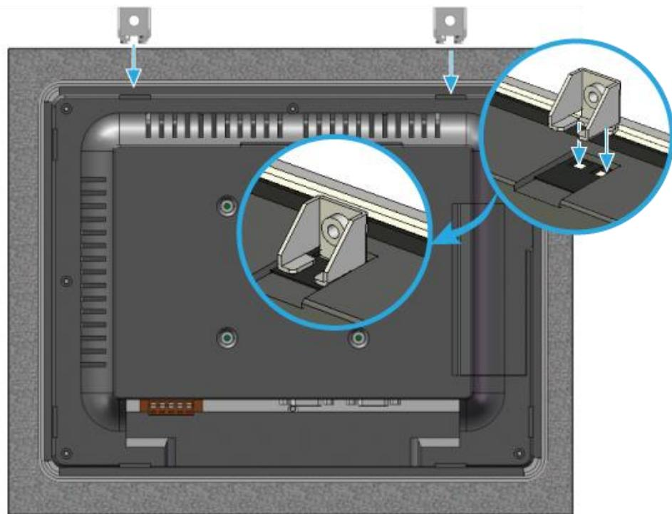
**Step 4: Screw the panel mounting clips to the panel.**
