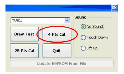
4.4. Touch the "X" icons on the monitor one by one to perform the calibration process.
