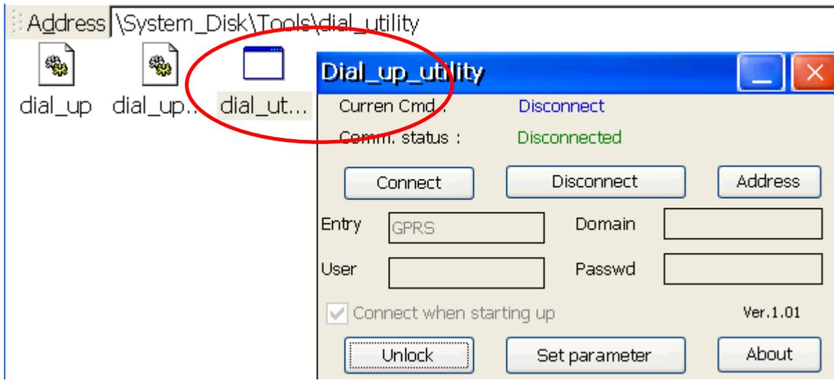
Step 2: Click the "Unlock" button and then enter the name for VPN connection, the User ID, and the password in the textbox and check the "Connect when starting up" checkbox. Click the "Lock" button to complete settings.
