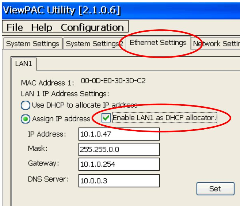
Step 2: Set a static IP address and a Mask for LAN1. The ViewPAC will then allocate the IP address to each device (i.e., if you set the Mask to 255.255.0.0, the ViewPAC will allocate the IP address 10.1.x.x. If you set the Mask to 255.255.255.0, the ViewPAC will allocate the IP address 10.1.0.x, where x=0 to 254).
