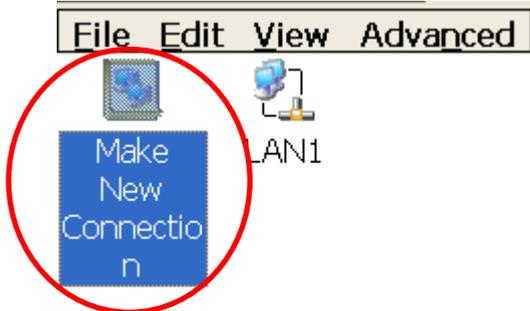
Step 3: In the "Make New Connection" dialog box, enter a name for the connection and select either the "PPTP" or the "L2TP" option as the connection type, and then click the "Next" button.
