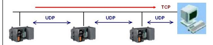
The following PAC support "IO connection > UDP" to use "UDP\_send" and "UDP\_recv" to deliver UDP data between PACs (or between PAC and PC).
