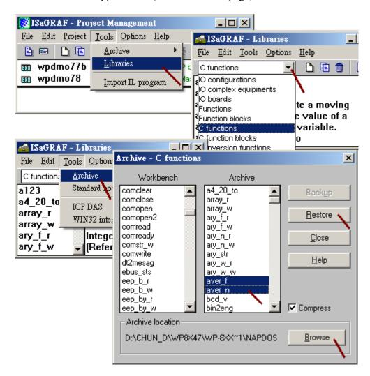
The demo program "wpdmo81.pia" can be obtained from the FAQ-120. It uses the hardware WP-8xx7 plus one i-8017HW in its I/O slot 1(Note: the leftmost I/O slot No. of the WP-8xx7 is 0). Please set the jumper of the I-8017HW to "single-end" and refer to the FAQ-039 for using ISaGRAF Variable array.
