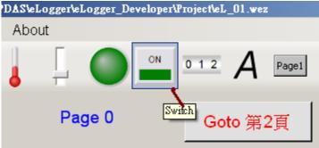
Set Tag Type as "DO Tag", Tag Name as "DO $_102$ ", ConfirmWindow as "True" (will output after confirmation), MouseControl as "True" (True: allow Tag outputs its value; False: read only, not allowed to output). Then setup the Text and color you want.
