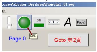
This "LED" is to control the ISaGRAF variable OUT\_101 (the relative DO Tag in eLogger is DO\_101). Please set Tag Type as "DO Tag", Tag Name as "DO\_101", ConfirmWindow as "True" (will output after confirmation), MouseControl as "True" (True: allow Tag outputs its value; False: read only, not allowed to output). Then setup the Text and color you want.
