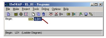
We are going to create a "SYSTIM\_R" function block to get the PAC 's Hour/Minute/Second . Click "Block on the left", then double click inside the block to select the "SYSTIM\_R" .
