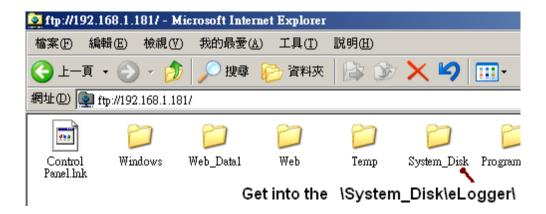
Then click "My Device" on the VGA of the controller, get into the "\System\_Disk\eLogger\" path, then run "eLogger.exe". Check "Auto Run" and exit it.
