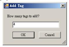
Then click the first tag to key-in the Tag Name as "Long\_1", Memory Add as 1, Data Type as "32-bit Signed Long", Gain as 1 and Offset as 0.
