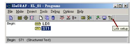
To download project via Ethernet cable, please select "ETHERNET" and enter the IP address of the PAC and must set Port number as 502.
