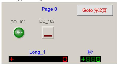
Then by the similar way, add a "Seven Segment" component with Tag Type as "AO Tag", Tag Name as "Float\_5", MouseControl as "True" (True: allow Tag outputs its value; False: read only, not allowed to output), DigitalNumber as 7 and "Decimal" as 2 (display 2 decimal places). The range that operator can input is  $-1000 \sim +1000$ , so please set its "Output Limit(Max)" as 1000 and "Output Limit(Min)" as -1000.
