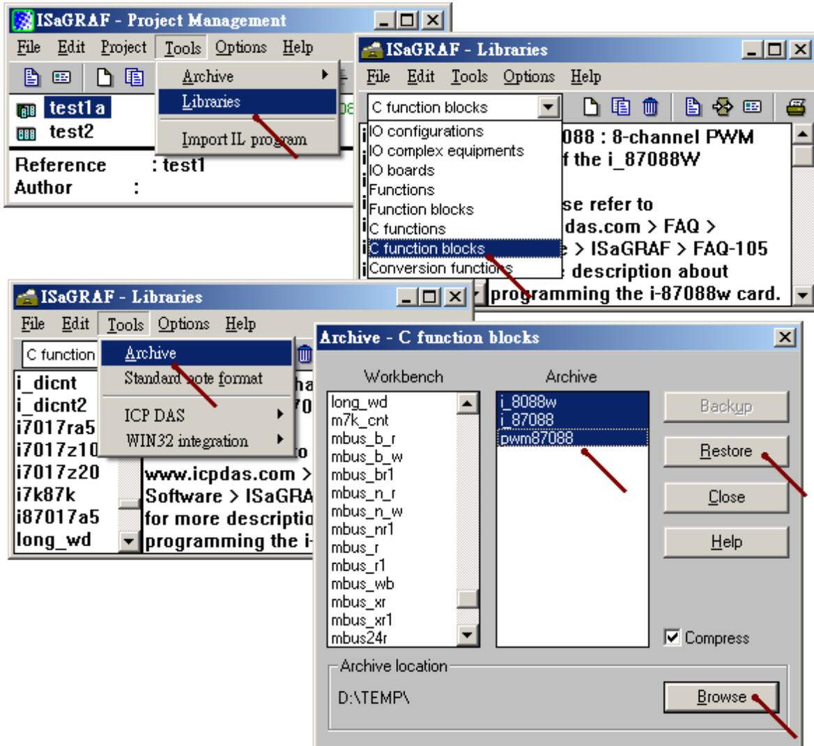
Install the I/O complex-equipments - "i\_87088w" :
