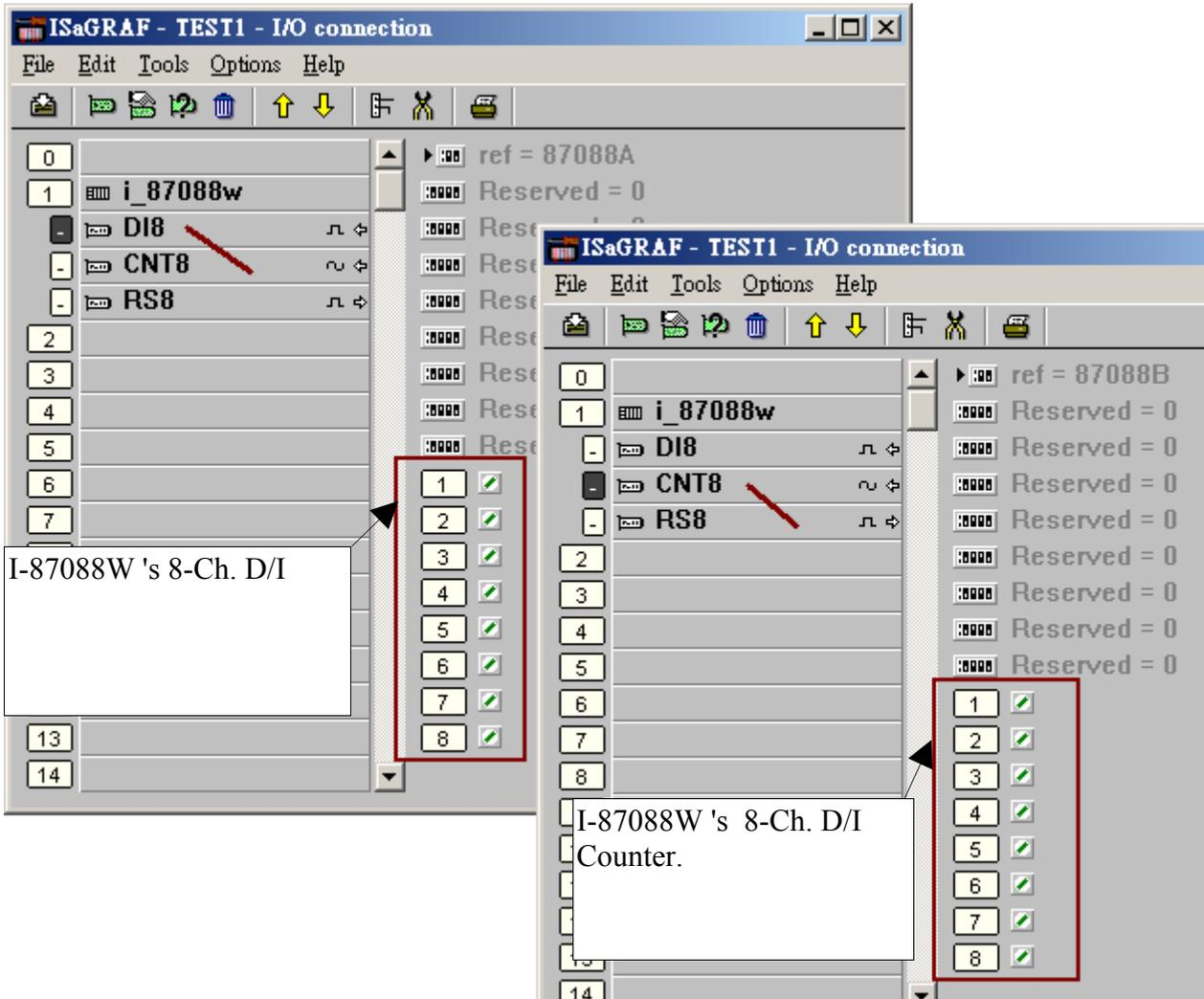
Then using the c-function block “pwm87088” to control the PWM output for each channel.
