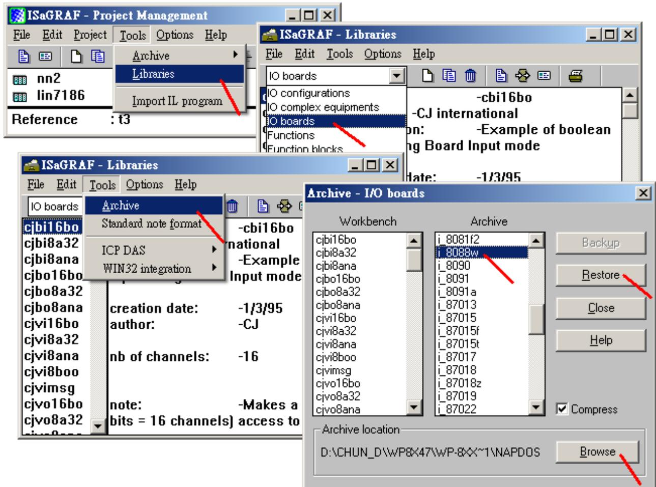
Install the c-function block - "i\_8088w", "i\_87088" and "pwm87088" :
