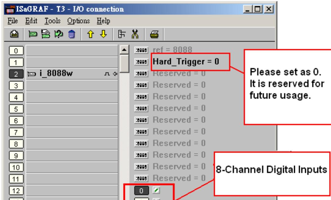
Then using the c-function block “i\_8088w” to control the PWM output for each channel.
