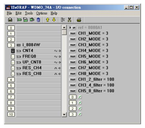
The default "CHx\_x\_filter" setting is 0. It is for filtering, the input signal with smaller time-width (that is, larger input frequency) will be filtered out. (Can be 0, 1 to 32767, unit is 0.001 ms)
