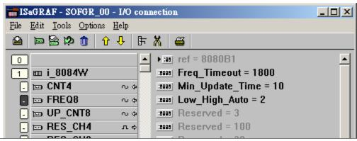
For example, setting "Freq Timeout" as 100 ms. If no signal wave
