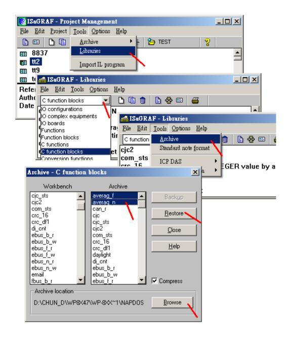
Then you may refer to the "wdmo\_74e" project to test these two function blocks. The sampled number (parameter "N\_") can be 1 to 20 only for iP-8xx7 and uPAC-7186EG . While "N\_" can be 1 to 50 for WP-8xx7 (driver 1.18 or later) and VP-2xW7(driver 1.09 or later) and W-8xx7(driver 4.18 or later). The interval setting (parameter "TIME\_") can be T#0s or T#10ms to T#1h. Setting as T#0s means to sample and calculate once at each calling. (Normally, this means in every PLC scan).
