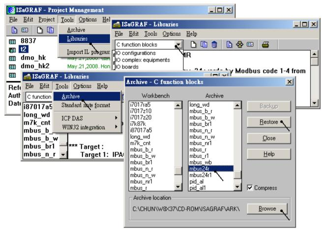
Then program the "Mbus24r" and "Mbus24r1" in the Ladder or Function Block program. Its usage is similar as the "mbus\_r" and "Mbus\_r1". Please refer to the Chapter 8 of "ISaGRAF User's Manual" or the "user\_manual\_i\_8xx7.pdf" and "user\_manual\_i\_8xx7\_appendix.pdf" at the following location.
