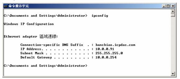
Then please fill-in this Gateway IP address to your wincon's Ethernet port setting (If controller model is W-8347/8747, you can enable two Ethernet ports, then you need to fill-in both with the same Gateway IP)
