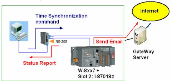
If the PC resides at the Internet, it must use a fixed Internet IP. And also please modify the initial value of the "IP\_correct\_PC" variable and modify the IO connection – udp\_ip – "to\_ip1" value in the ISaGRAF project "wdmo\_65b" to be the same as that Internet IP. Then re-compile it.
