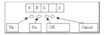
Press the "Up" or "Down" buttons until "y" appears in the LED readout then press the "OK" button. This will delete the currently installed ISaGRAF project from the controller system. After that press some "Cancel" to exit the hardware setting.
