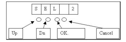
Press the "Up" or "Down" buttons until "dEL" appears in the LED read out.
