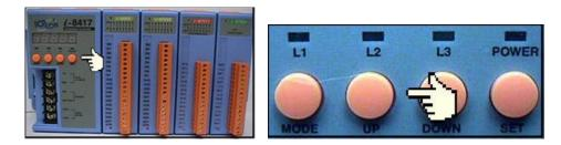
When the first display appear, press the "Up" or "Down" button until "SEL 2" (Select 2) appears in the LED readout.
