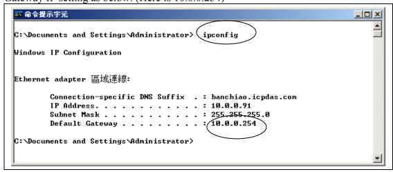
Then please fill-in this Gateway IP address to your controller's Ethernet port setting (If controller model is W-8347/8747, you can enable two Ethernet ports, then you need to fill-in both with the same Gateway IP)
