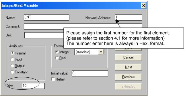
And then using "S\_MB\_ADR" to assign the other network address number for each element. For example,
