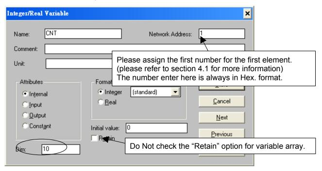
For example, setting integer variable array CNT[0..9] as retained data in the integer retained memory starting from 20 , 21 , ... to 29.
