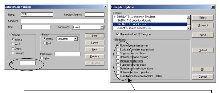
If using "Variable Array" in the program, please DO NOT check the 2nd, 7th, 8th and 9th Optimizer options, or the value of the Variable array will be incorrect. Recommend to check only the 1st – "Run two optimizer passes" option.
