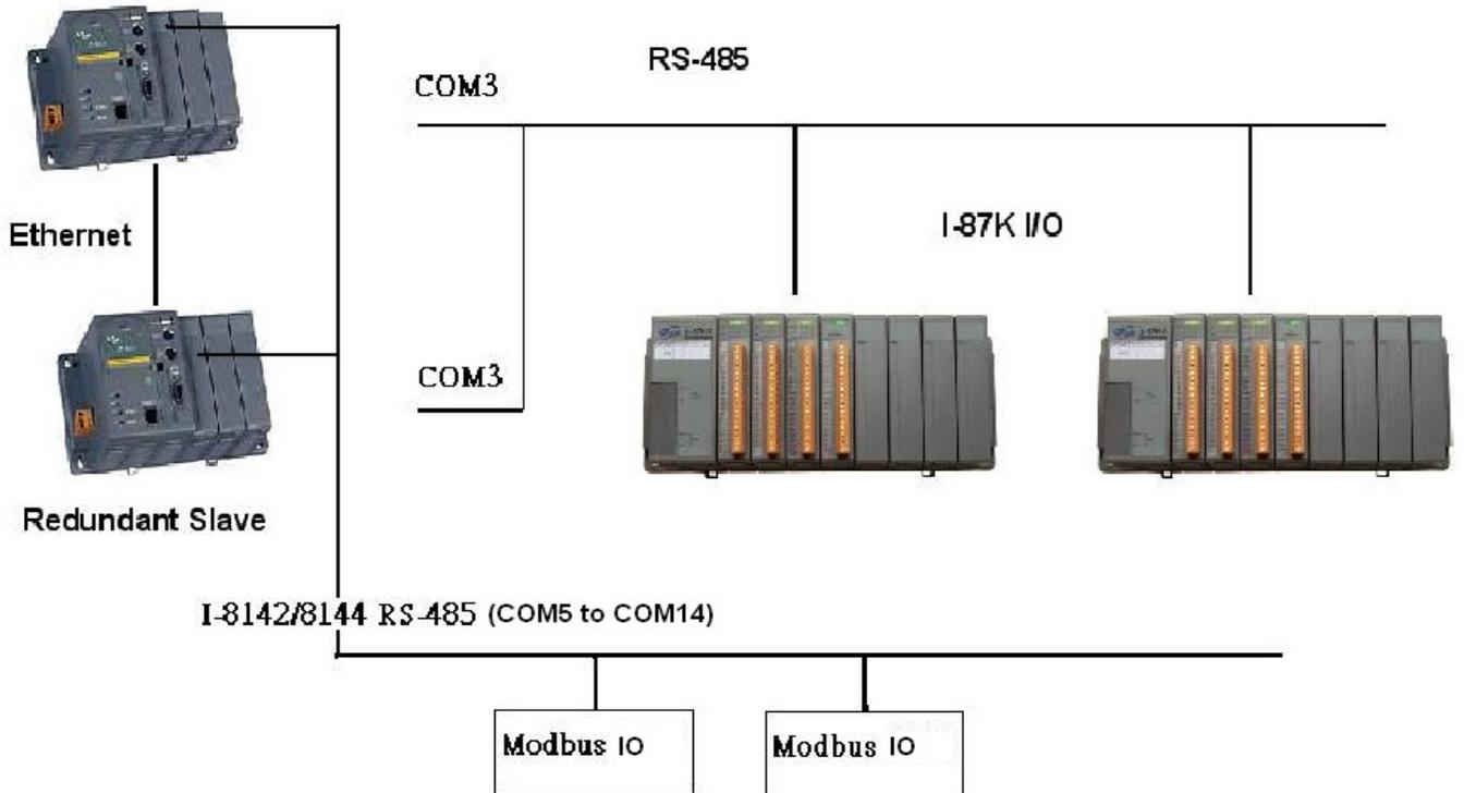
Please place Mbus\_xxx function blocks on the third position as below. Please refer to Chapter 8 for using Modbus RTU devices.
