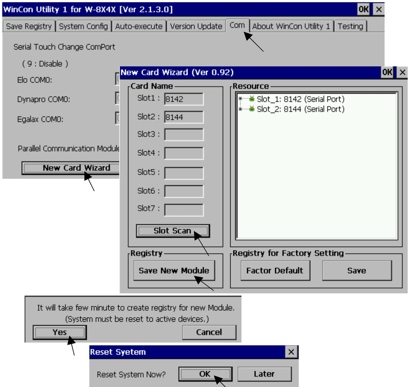
After the configuration succeed. The COM port No. for the expansion board is COM5 to COM14 in the ISaGRAF definition.
