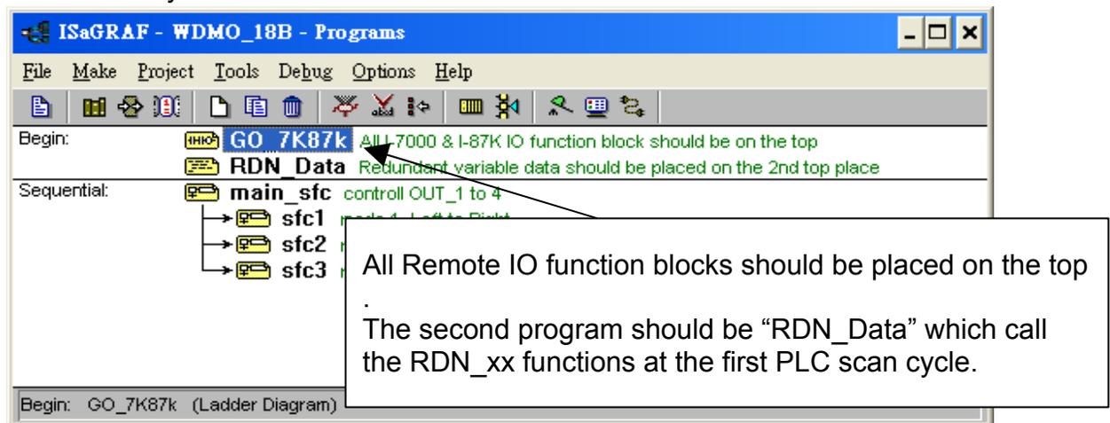
All redundant synchronous data should be set in the first PLC scan cycle by using the following functions. However not necessary for the digital inputs & analog inputs in slot 1 to 7 or in the RS-485 I-7K & I-87K IO ,they are automatically updated. Only the output and other important internal data should be set as synchronous data.
