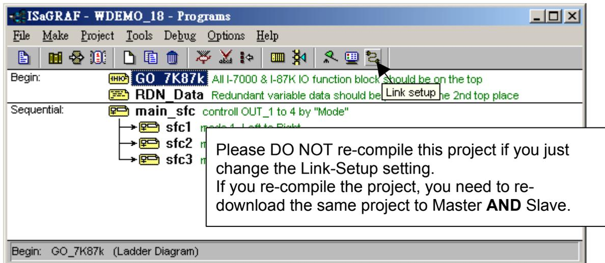
Please connect "rdn" in the IO connection window first as below. Please set the correct Master IP address and Slave IP address. For W-8x47, it is better to use IP address of the "LAN2" port. Please set "Remote\_IO\_type" to 1 if the remote IO is I-87K and I-7000 RS485 IO (**At least one Remote IO should be connected in COM3:RS485 when type=1**). (type 2 is reserved for future Modbus TCP/IP IO, not available before June.30,2006)
