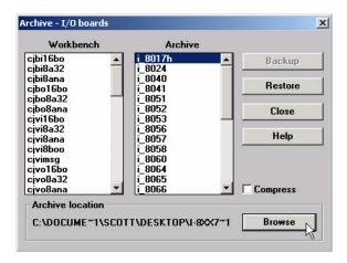
The drivers for the I-8xx7 control boards now appear in the "Archive" list box. Select all the required I-8xx7 I/O boards, and then click on the "Restore" button. The selected drivers will now install into the ISaGRAF.
