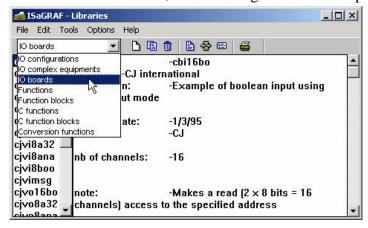
Select "IO Boards" (IO complex equipments, c functions or c function blocks as you need) from the drop down menu just below the file menu bar. Next, select the "Tools" option from the main menu bar, then select "Archive" from the file menu bar as shown below.
