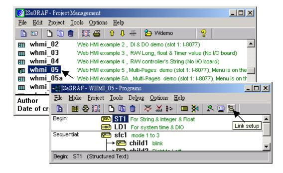
Click on "Setup" first and then entering the IP address of your controller. The port number should be 502.
