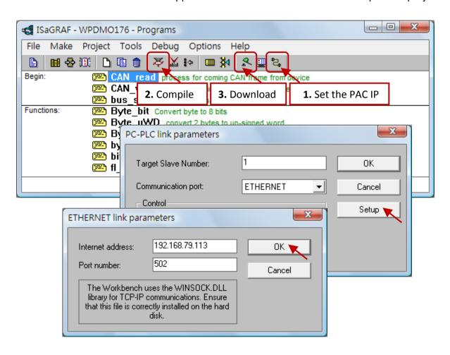
3. Click the menu bar "Debug" or tool button to download the "wpdemo176" project. After downloading this project, the "Debugger" window will show as the figure below.
