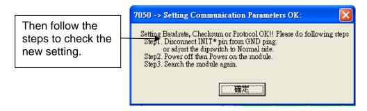
**Note:** Remember to remove the connection of I-7000's INIT\* and GND after the setting is
