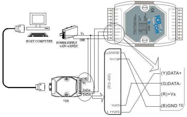
**Note**: For configuring I-7000 and I-87xxx I/O module, you have to prepare an I-7520R converter. For other wiring diagram please refer to "DCON Utility User's Manual".
