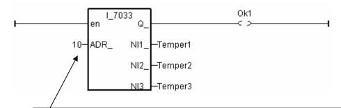
ADR\_ = 10 (TT=00, RR=00, AA=0A, Hex.) means "standard setting", address=10, the temperature input value is normally -32768 to + 32767
