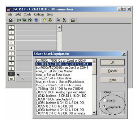
In the example provided, set the slot below number 9 to "Bus7000b: Remote".
