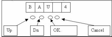
You can now change the baud rate setting by pressing the "UP" or "Down" button to the desired baud rate setting. The settings for the baud rate are as follows: (-) Disable COM (0) 1200, (1) 2400, (2) 4800, (3) 9600, (4) 19200, (5) 38400, (6) 57600, (7) 115200, (8) 300 & (9) 600. Press "OK" to save the selected setting. And then press some "Cancel" to exit the hardware setting.
