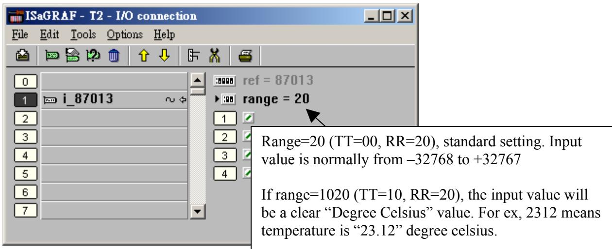
If setting range as 20 (or 21 to 2F), then it is “standard setting”. The temperature input value is 2’s compliment value from -32768 to +32767 depends on the “range” value. For example, setting range as 20, value of -32767 means temperature is about -100 Degree, +32766 is about +100 Degree. Value of 16383 means +50 Degree (**Note:**Normally value of -32768 or +32767 means wire “broken-line”)
