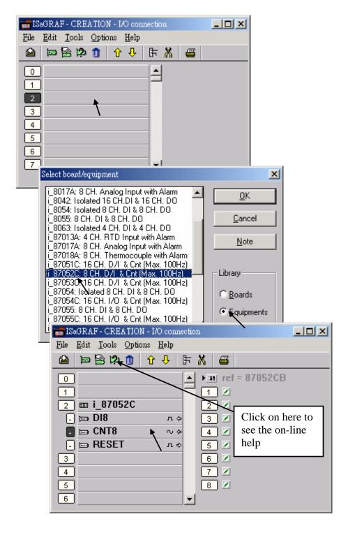
If the I-87xxx D/I Module is plugged in the 87K4, 87K5, 87K8 & 87K9 extension base module, or the I-7000 D/I module is used, Please refer to Chapter 6 to use "7000 utility" to set the appropriate address, baud rate , then connect "Bus7000" on the "I/O connection" window.
