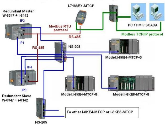
Wincon-8347 redundant system can connect max. 24 nodes of i-8KE4/8-MTCP I/O
