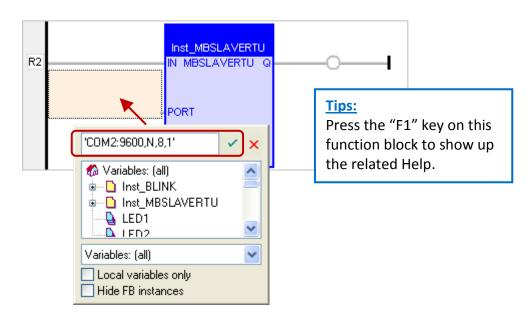
4. Double-click the left side of the "SLV" and then enter "1" (the value set in the Section 3.1 - Step 3), then click to finish the setting.
