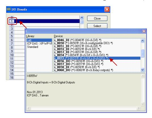
3. Click the "Close" button to exit the "I/O Boards" window. Note: Click the "Virtual/Real" button to change to the Virtual I/O (for testing) or the Real I/O. (The Real I/O is used in this example).
