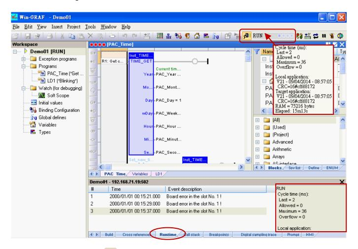
When doing the "On Line" ( ) operation, it will automatically switch to the "Runtime" tab and you can see if there is any error message for the downloaded program. (E.g., in this example, we need to plug the I-8055W module in the Slot1 of the PAC, and the message "Board error in the slot No. 1!" means there is no I/O module in the Slot1 or an I/O exception.)
