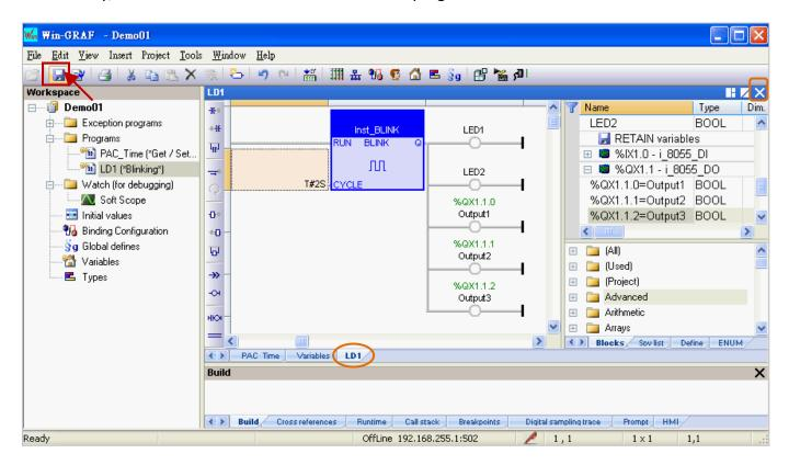
**Note**: """ means this program is opened (locked, cannot be deleted). Click the "X" in upper-right corner of window to close this program (un-locked, " ").
