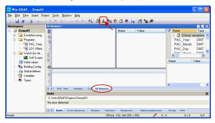
2. Click the "Insert Configuration" button on the left side of the "I/O Drivers" window and then select the "MOSBUS Slave" and click "OK" to enable a Modbus TCP Slave.
