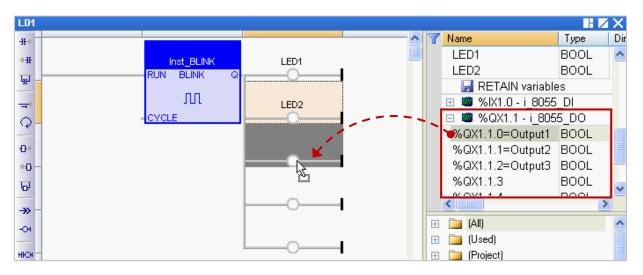
9. Mouse double-click on the left of the "CYCLE" and enter "T#2S" (to blink every two seconds), and then click to finish the setting.
