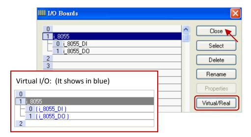
After linking the "i\_8055" I/O board, it will automatically add 8 input & output variables in the "Variables" window.
