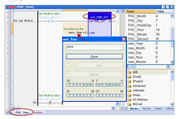
2. Set the "Set new time" variable to "TRUE" to write the new system time.
