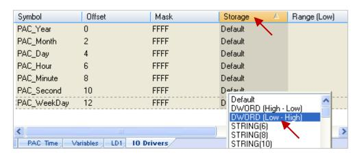
To expand this "Data Block" and you can see the Modbus addresses of all variables. It equals to the "Offset" value plus 1 (Base address).
