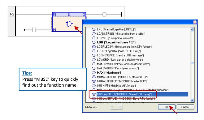
3. In the "MBSLAVERTU" function block, mouse double-click the left side of the "PORT" and enter a string 'COM2:9600,N,8,1' (it means using the Win-GRAF PAC's COM2 to communication with the Modbus Master) and then click to complete the settings.
