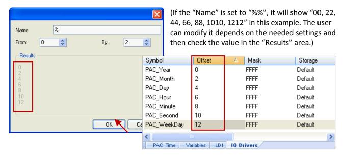
9. Click "Storage" to select entire columns and then press "Enter" key to display a drop-down menu. Then, select "DWORD (Low – High)" and press "Enter" key to complete the setting. (If using a 16-bits or below, it's no need to set the "Storage" item.)
