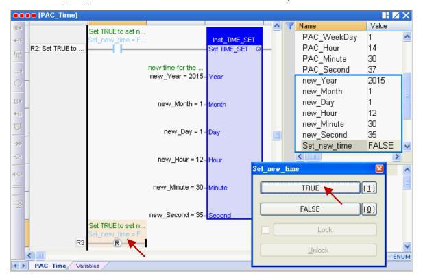
3. Then, the new system time will show on the "TIME\_**GET**" function block (or the Variables Area), and the "Set new time" variable will be reset to "FALSE" automatically.
