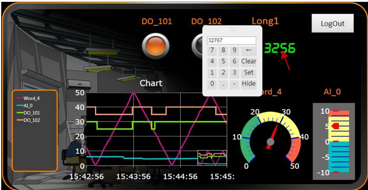
Note: To test negative value, first set the Long1 as a negative value on the local HMI page on PAC.
