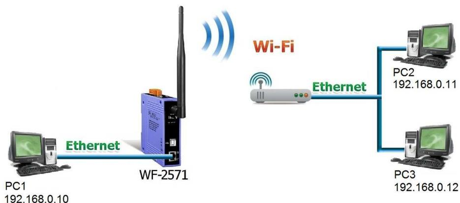
Figure 7: AP connection test architecture
