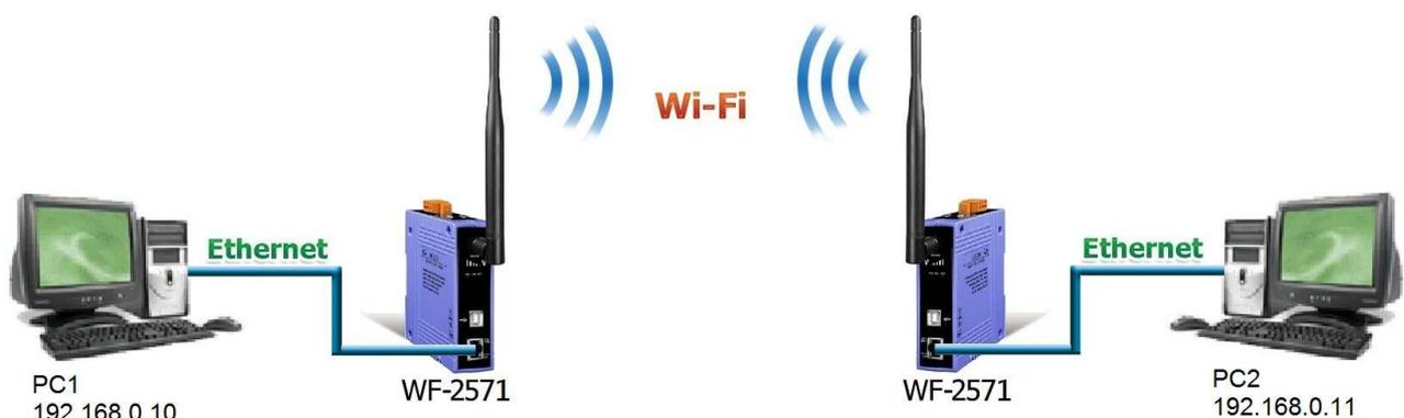
Figure 2: Ad-Hoc connection test architecture
