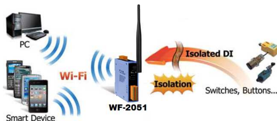
Figure 4-1: WF-2051 + Laptop application architecture
