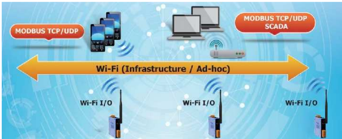
Figure 1-1: Application architecture for the WF-2000 series
