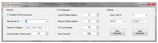
Figure 3-5: Pair connection configuration screen
