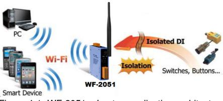
Figure 4-1: WF-2051 + Laptop application architecture
