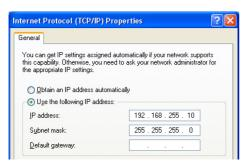
Figure 7: IP configuration interface
