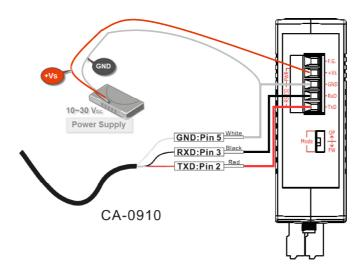
Figure 2-8 Power and Serial port wire connection
