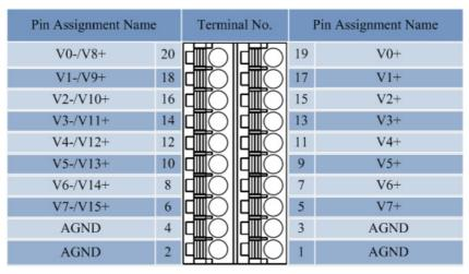
Figure 2-3 I/O Connector of WF-2017
