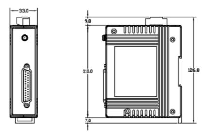
Figure 2-5 Front / Left Side dimension of the WF-2019
