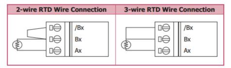
Figure 2-9 AI wire connection of WF-2015
