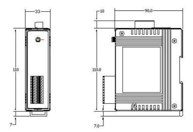
Figure 2-4 Front / Left Side dimension of the WF-2015/WF-2017/WF-2026
