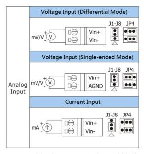
Figure 2-13 Al wire connection of WF-2017
