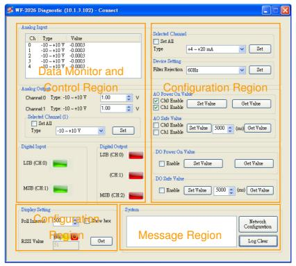
Figure 3-7 WF-2026 diagnostic screen
