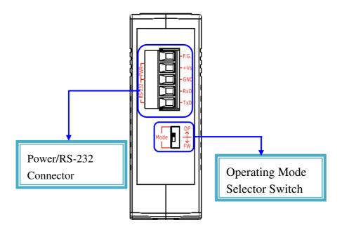
Figure 2-3 Top Panel of the WF-2000
