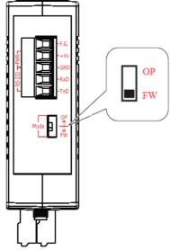
Figure 2-11 FW Position of Dip-Switch
