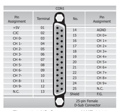
Figure 2-4 I/O Connector of WF-2019
