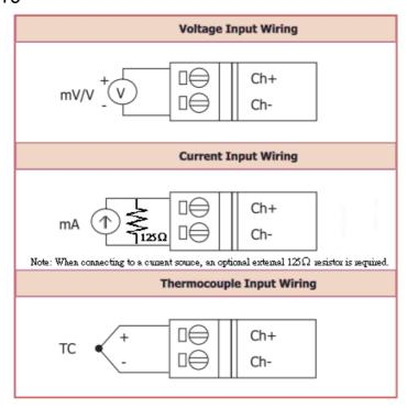
Figure 2-14 Al wire connection of WF-2019
