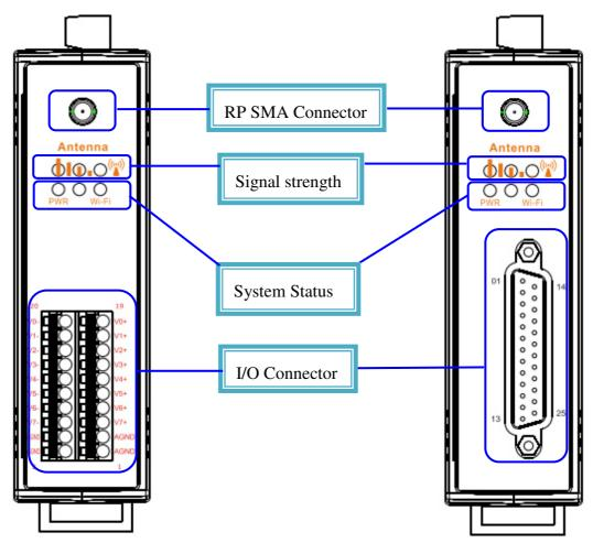
Figure 2-1 Front Panel of the WF-2000 AIO modules
