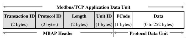
Figure 5-1 Modbus/TCP Application Data Unit
