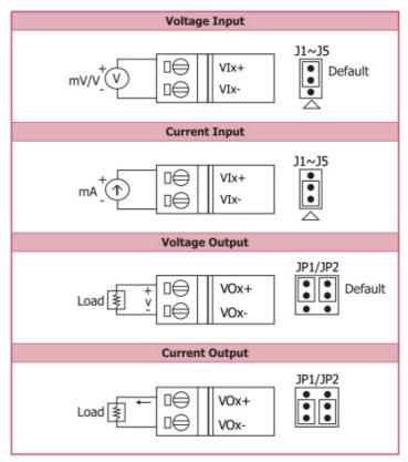
Figure 2-15 AIO wire connection of WF-2026
