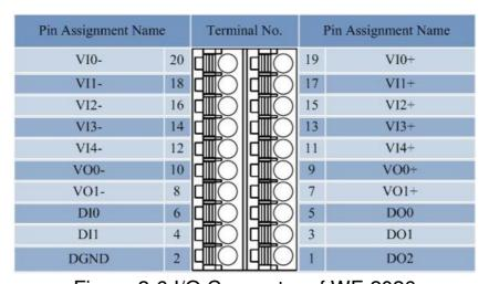
Figure 2-6 I/O Connector of WF-2026
