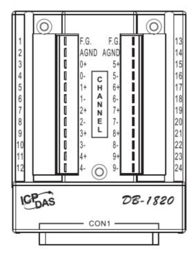
Figure 2-5 Pin Assignment of DB-1820
