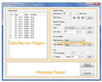
Figure 3-6 WF-2019 diagnostic screen
