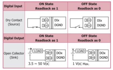
Figure 2-16 DIO wire connection of WF-2026
