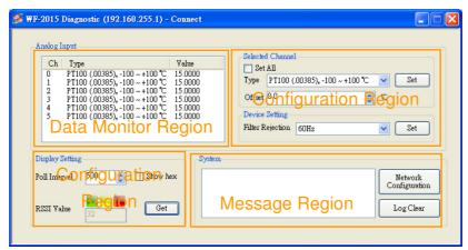
Figure 3-4 WF-2015 diagnostic screen
