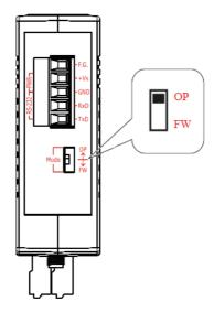
Figure 2-15 OP Position of Dip-Switch
