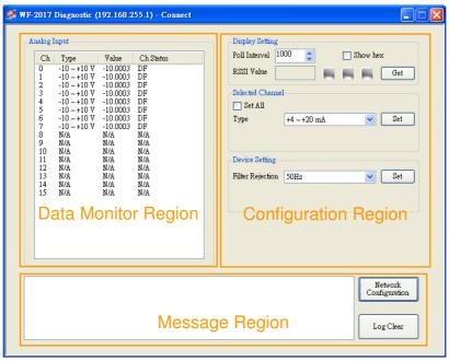
Figure 3-5 WF-2017 diagnostic screen
