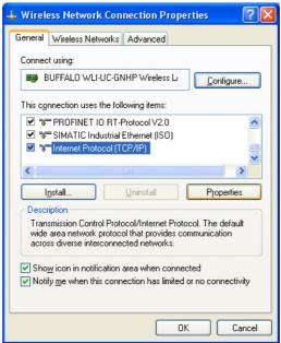
Figure 4-4 Properties setting of Internet Protocol (TCP/IP)
