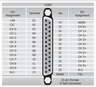
Figure 2: Pin Assignment of D-Sub 25-pin
