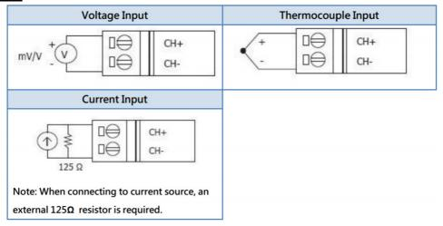
Figure 5: Wire connections
