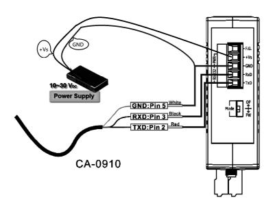
Figure 4: Power and Serial port wire connection
