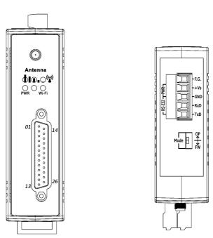
Figure 1: Appearance of the WF-2019
