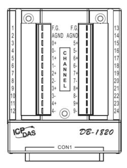
Figure 3: Pin Assignment of DB-1820
