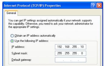
Figure 7: IP address configuration interface
