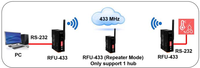
PC cannot monitor the thermometer and hygrometer directly because the distance is too far. But the repeater can bypass the RF message one side to another and let PC can monitor the thermometer and hygrometer.
