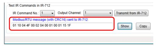
Fig. 13: Test IR commands stored in IR-712
