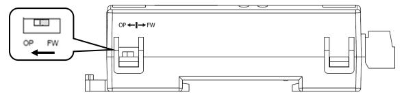
Fig. 2: Push DIP switch to OP position
