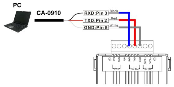
Fig. 3: Serial wire connection between IR-712 and PC
