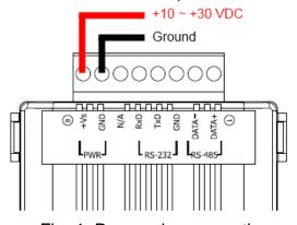
Fig. 4: Power wire connection
