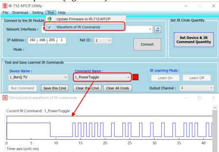
**Figure 3-22** *Opened waveform window shows current IR command.*
