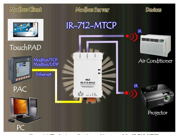
Figure 1-1 The basic application architecture of the IR-712-MTCP.
