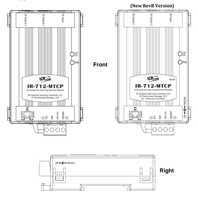
Figure 2-1 The appearance of the IR-712-MTCP
