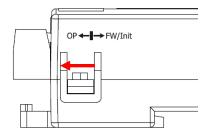
Figure 2-9 DIP switch (OP mode)
