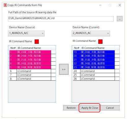
Figure 3-20 Copy IR commands to current device.
