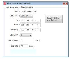
**Figure 3-5** *The basic settings of the IR-712-MTCP.*
