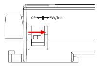
Figure 2-8 DIP switch (FW/Init mode)
