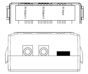
Figure 2-2 IR output 3.5 mm audio jack
