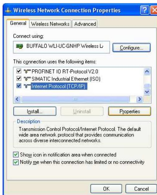
Figure 4-5: Properties setting of Internet Protocol (TCP/IP)
