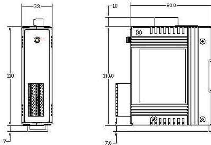
Figure 2-6: Front / Left Side dimension of the WF-2017
