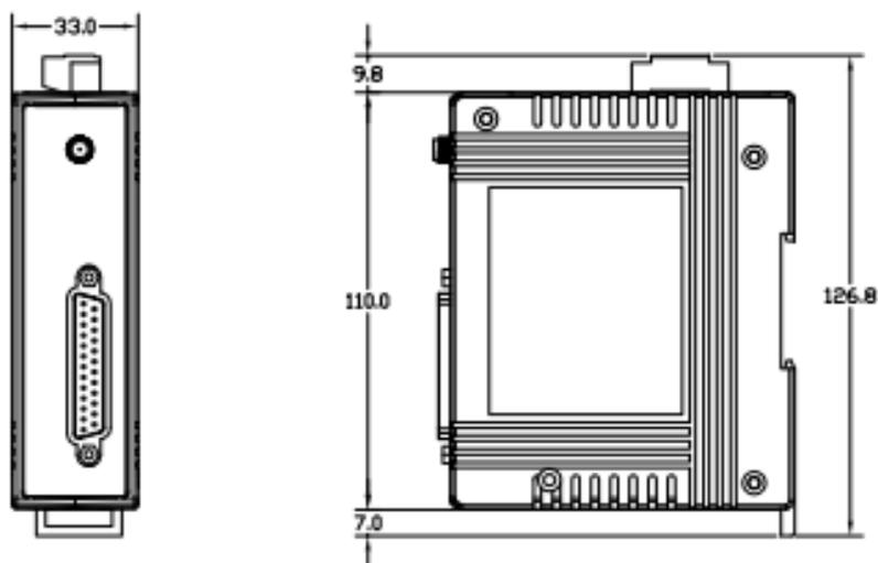
Figure 2-7: Front / Left Side dimension of the WF-2019
