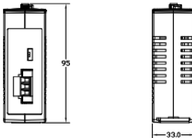
Figure 2-9: Top / Bottom dimension of the WF-2019
