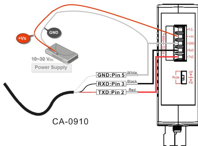
Figure 2-10: Power and Serial port wire connection
