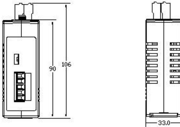
Figure 2-8: Top / Bottom dimension of the WF-2017
