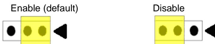
Figure 2-13: Watchdog timer Jumper Position
