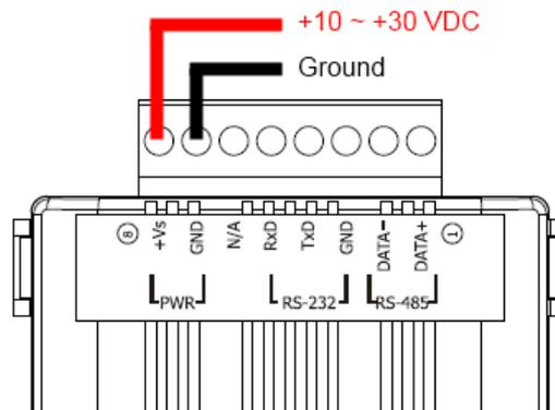
Fig. 4: Power wire connection
