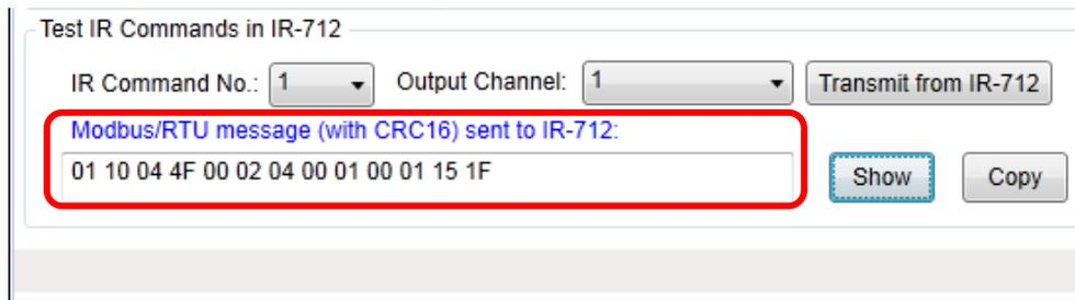
Fig. 13: Test IR commands stored in IR-712
