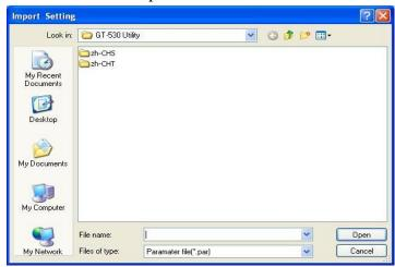
B. Export Parameters: The function is used for saving the setting of "Device parameter" window as .par file. When press "Export" button, a file selection window would pop-up for users to save the setting as .par file in specific path.
