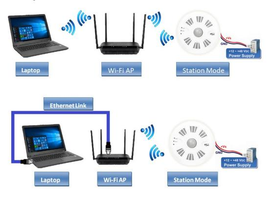
The PIR-230-WF device can be configured as AP mode, such that the PC/Laptop can be connected through Wi-Fi directly. Only one device is allowed to be connected to the PIR-230-WF module in AP mode.
