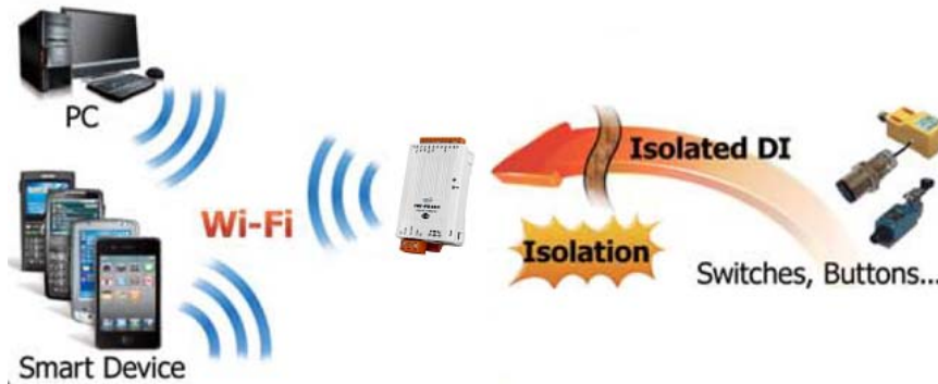
Figure 4-1: tWF + PC/Laptop/Smart Device application architecture
