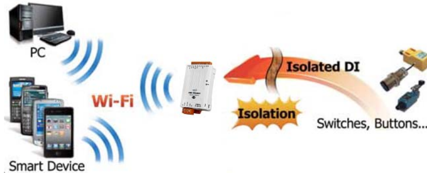
Figure 4-1: tWF + PC/Laptop/Smart Device application architecture
