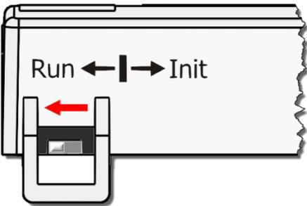
**Step 4** Reset the Init/Run switch on the tSH-700 module to the "Run" position and reboot the device.
