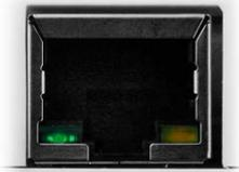
The tSH-700 module is equipped with an RJ-45 jack that is used as the 10/100 Base-TX Ethernet port and features networking capabilities. When an Ethernet link is detected and an Ethernet packet is received, the **Link/Act LED (Orange)** indicator will be illuminated. When power is supplied via PoE (Power-over-Ethernet), the **PoE LED (Green)** indicator will be illuminated.
