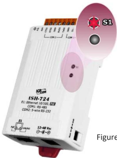
5. Verify that the System LED indicator is flashing.
