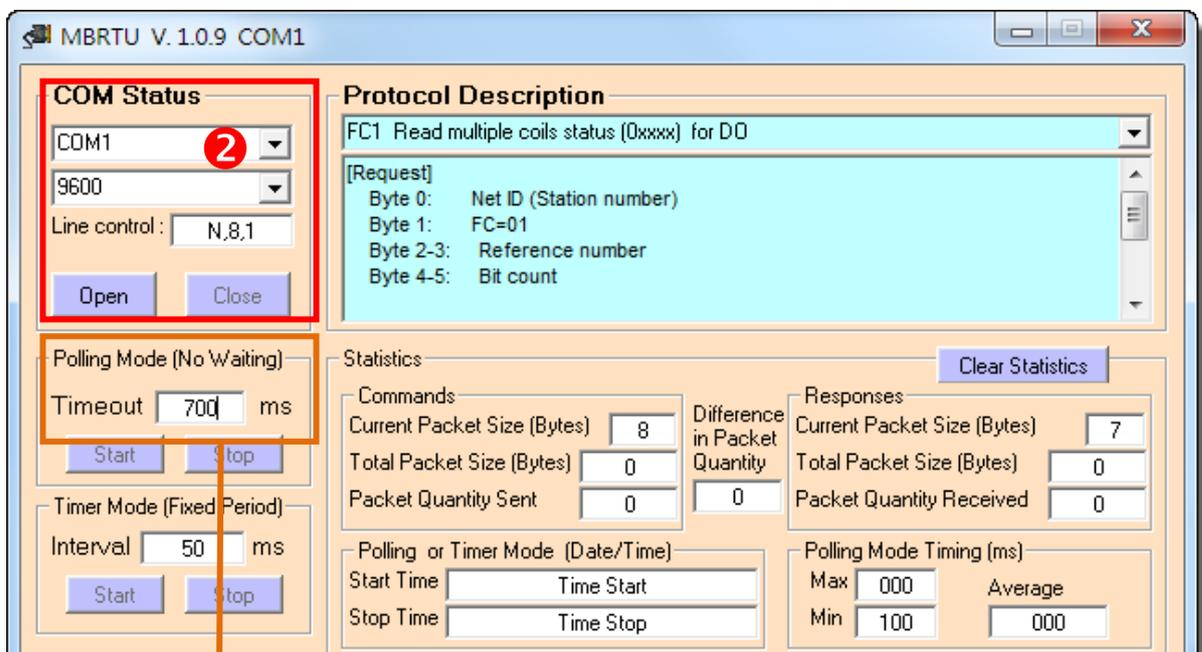
Please ensure that the Timeout value in the above window should larger than the Slave timeout setting in the tSH-700 series module.
