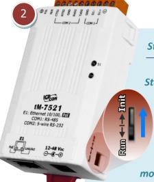
Step 2: Set the "Init Switch" to the "Init Mode" position.
