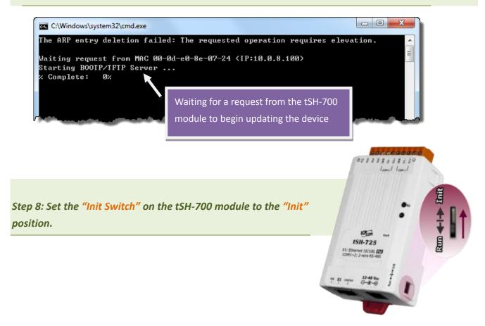
Step 9: Power-on reset the tSH-700 module in "Init Mode" to initiate the update.
