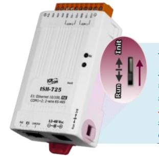
Step 2: Set the "Init Switch" to the "Init" position.
