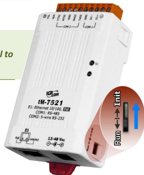
**Step 9: Power-on and reboot** the tM-752N module in **“Init Mode”** to initiate the update.
