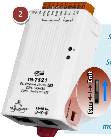
*Step 2: Set the "Init Switch" to the "Init Mode" position.*
